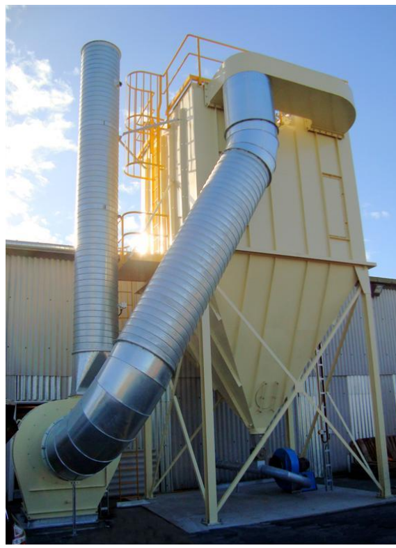
James Hardie Cement fibre board dust Pulse Jet Filters, complete with low pressure blowline
